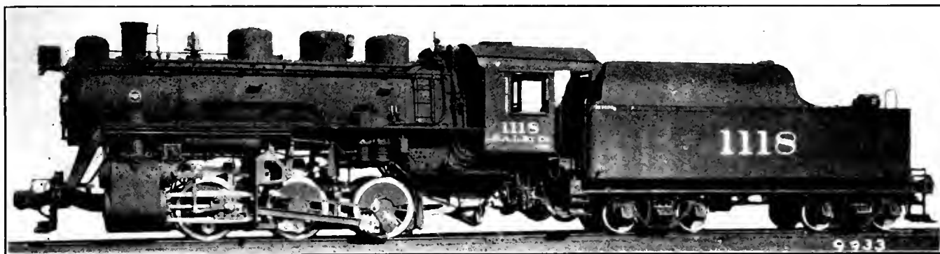
Six-Coupled Switching Locomotive of the Seaboard Air Line Built by the Baldwin Locomotive Works
